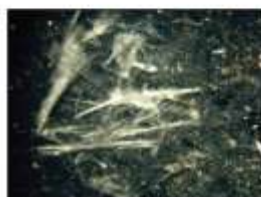
Asbestos fibres from vermiculite insulation
