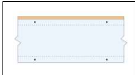
Figure 2b: side view of the installation of 12.5 mm (1/2 in.) regular gypsum board flange-to-flange of I-joist
