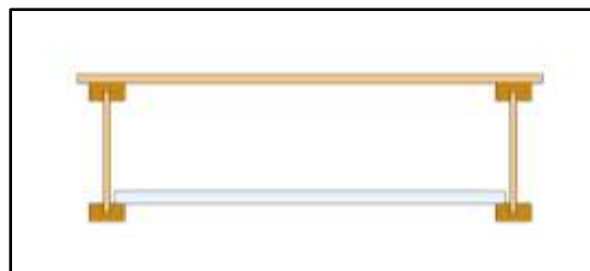
Figure 3a: end view for wood I-joist at 600 mm spacing, placing 15.8 mm (5/8 in.) regular gypsum board on top of bottom flange of I-joist
