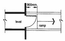
Practically however, depending on whether the ramp slopes up or down, there may be conflict between the ramp surface and the edge of the door swing, if the door is wider than the landing length. This situation is not addressed by the Building Code.
