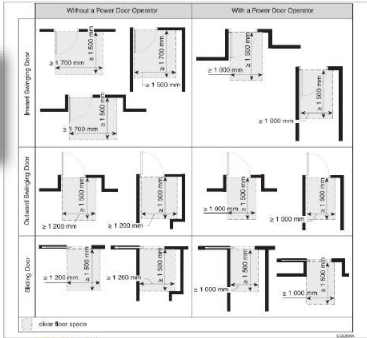
Figure A-3.8.3.6.(14) to (16) Minimum clear floor space required at doors in an accessible path of travel
