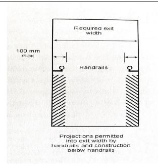
It is interpreted that handrails can project not more than 100 mm into each side of the required width of a stair.
